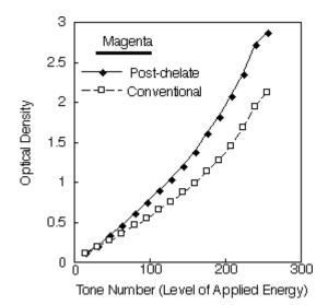
Fig. 5 Characteristic curves of Thermal Dye Transfer
