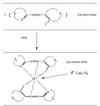
Fig. 4 Principle of post-chelate process
