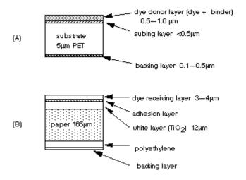
Fig.1 Dye donor sheet (A) and dye receiver sheet (B)
