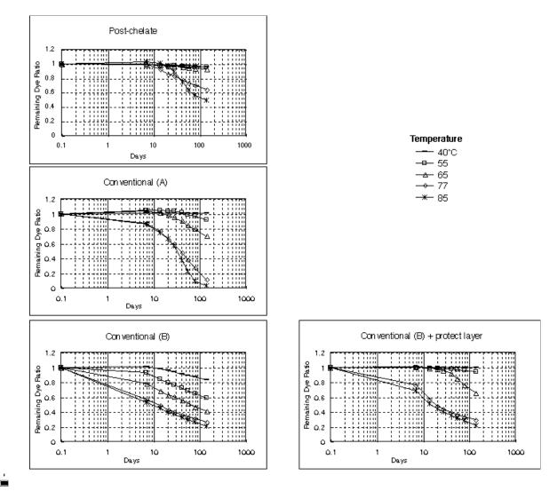
Fig. 7 Color fading by temperature (Cyan images)
